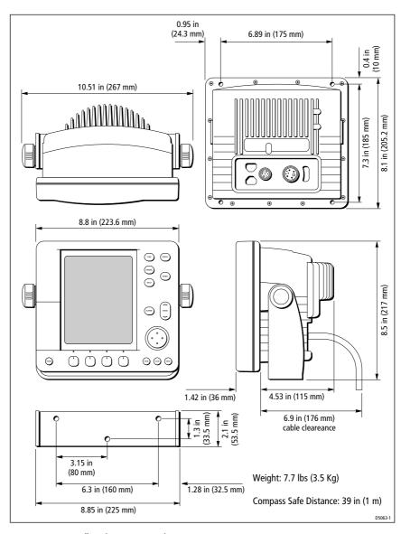
Figure 6-4: 7" Color LCD Display Dimensions
